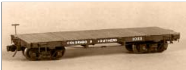
#29407 - DSP&P Flat/Gondola Car This basic 26' car was the most widely used on the system. This kit provides parts for any one of the following cars: flat car, lime car, lumber cars, log car or coal loader.
